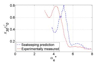
Figure 4: Comparison between experimental and predicted heave RAOs  $(H_{1/3} = 1.12m, T_0 = 8s, U = 38kts, (25mm, 1.2s, 2.98m/s model scale)).$
