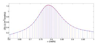
Figure 1: A JONSWAP wave spectrum illustrating the constant energy method of separating the spectrum into a series of regular waves. The dashed lines and points show the mid-point of each energy band, a regular wave of this frequency represents the energy within the associated band ( $H_{1/3} = 2.24m$ ,  $T_0 = 8s$ ).
