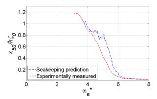
Figure 5: Comparison between experimental and predicted pitch RAOs  $(H_{1/3} = 1.12m, T_0 = 8s, U = 38kts, (25mm, 1.2s, 2.98m/s model scale)).$
