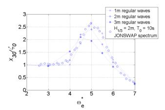
Figure 2: Numerical heave RAOs for a 112m wave-piercing catamaran. 1m, 2m and 3m regular waves (U = 38kts) compared with the response from a JONSWAP wave spectrum ( $H_{1/3} = 2.0m$ ,  $T_0 = 10s$ , U = 38kts).
