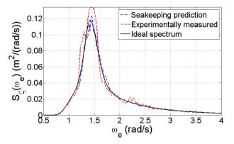
Figure 3: Encountered wave spectra (numerical and measured) compared with the ideal for a JONSWAP spectrum ( $H_{1/3} = 1.12m$ ,  $T_0 = 8s$ , U = 38kts, (25mm, 1.2s, 2.98m/s model scale)).
